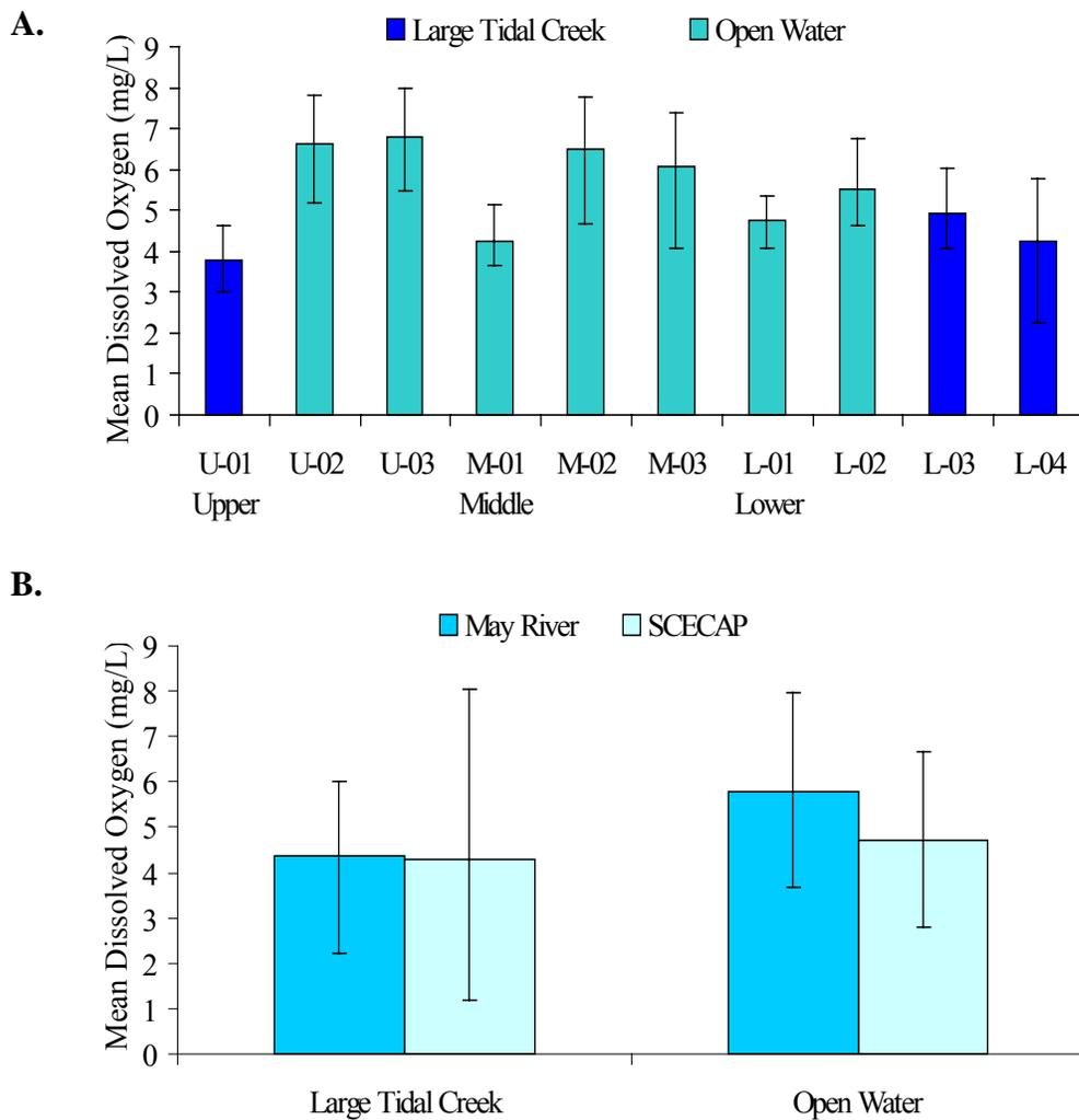
**Figure III-39. Mean bottom dissolved oxygen during the semi-continuous summer deployment from the May River large tidal creek and open water sites (A.), and compared to 2002 SCECAP stations (B.). Error bars represent 1 standard error.**
