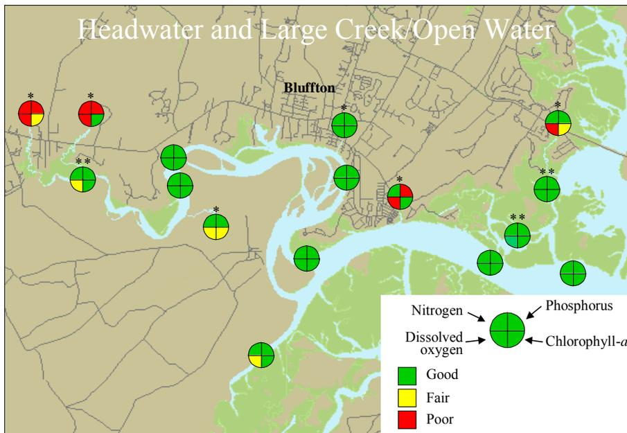
**Figure V-1. Summary of key water quality measures collected at the May River sites. Green represents no exceedances of standards established by SCDHEC (2001) or criteria used by the SCECAP program (Van Dolah and others, 2002). Yellow indicates at least one exceedance, and red indicates two or more exceedances. Sites with an \* represent headwater tidal creeks. Sites with \*\* represent large tidal creeks.**
