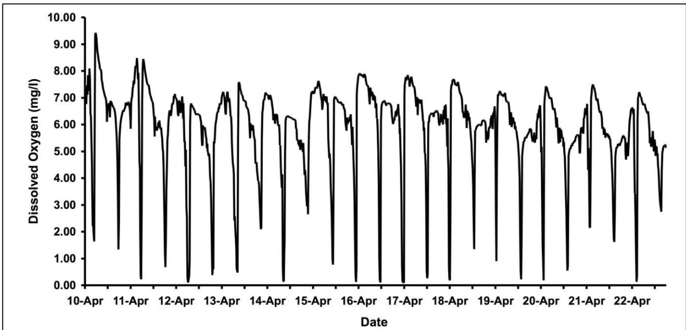
Figure 17. Dissolved oxygen levels recorded by a continuous data sonde deployed at the mouth of Rose Dhu Creek over two weeks in April 2008.
