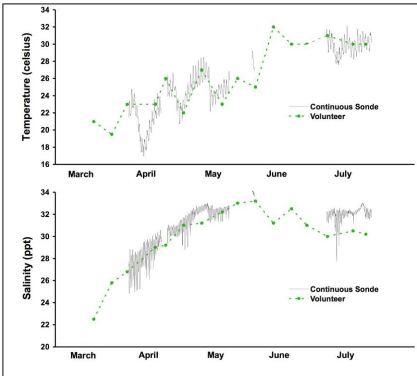
*Figure 20. Values for temperature and salinity compared between data collected by the Volunteer Monitoring network and by a continuous data sonde in Rose Dhu Creek between March and July 2008.*
