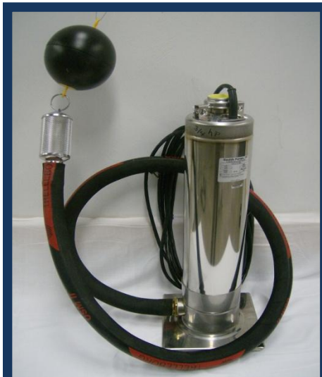
Figure 14. Submersible cistern pump with custom-made bottom intake attached to a floating filter.
