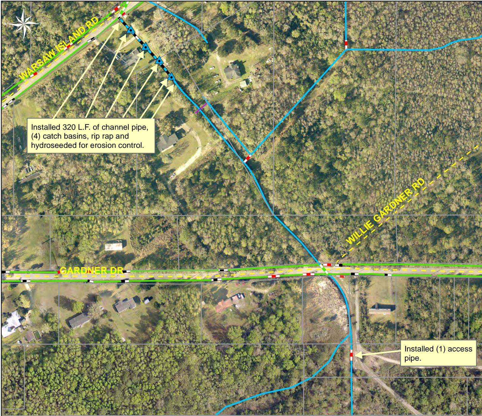
Installed 320 L.F. of channel pipe, (4) catch basins, rip rap and hydroseeded for erosion control.
