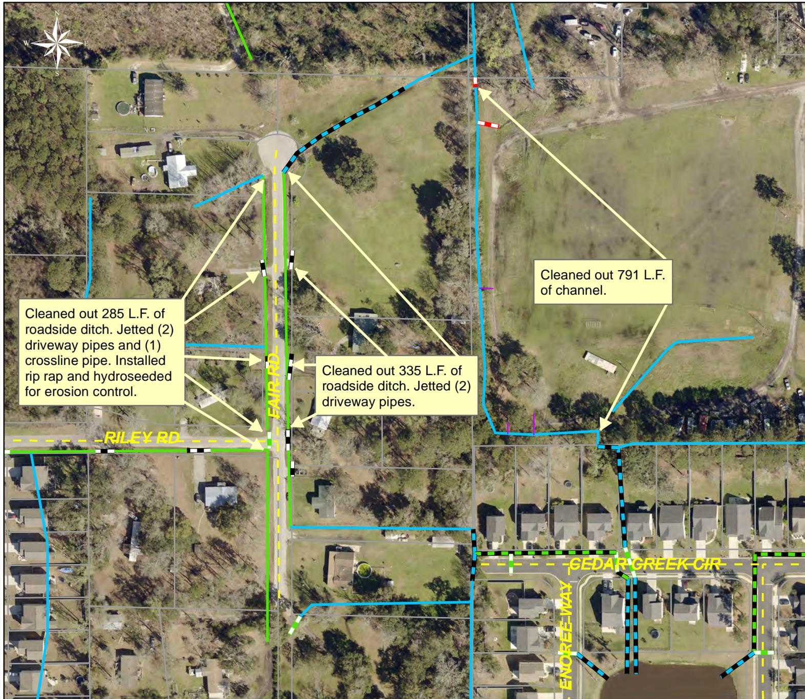
Cleaned out 285 L.F. of roadside ditch. Jetted (2) driveway pipes and (1) crossline pipe. Installed rip rap and hydroseeded for erosion control.
