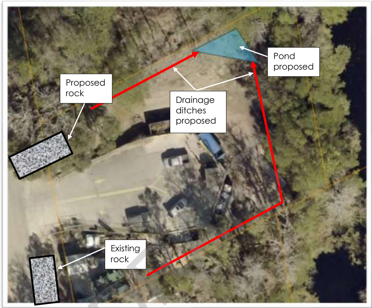
Figure 10 Pritchardville Retrofit Sketch
