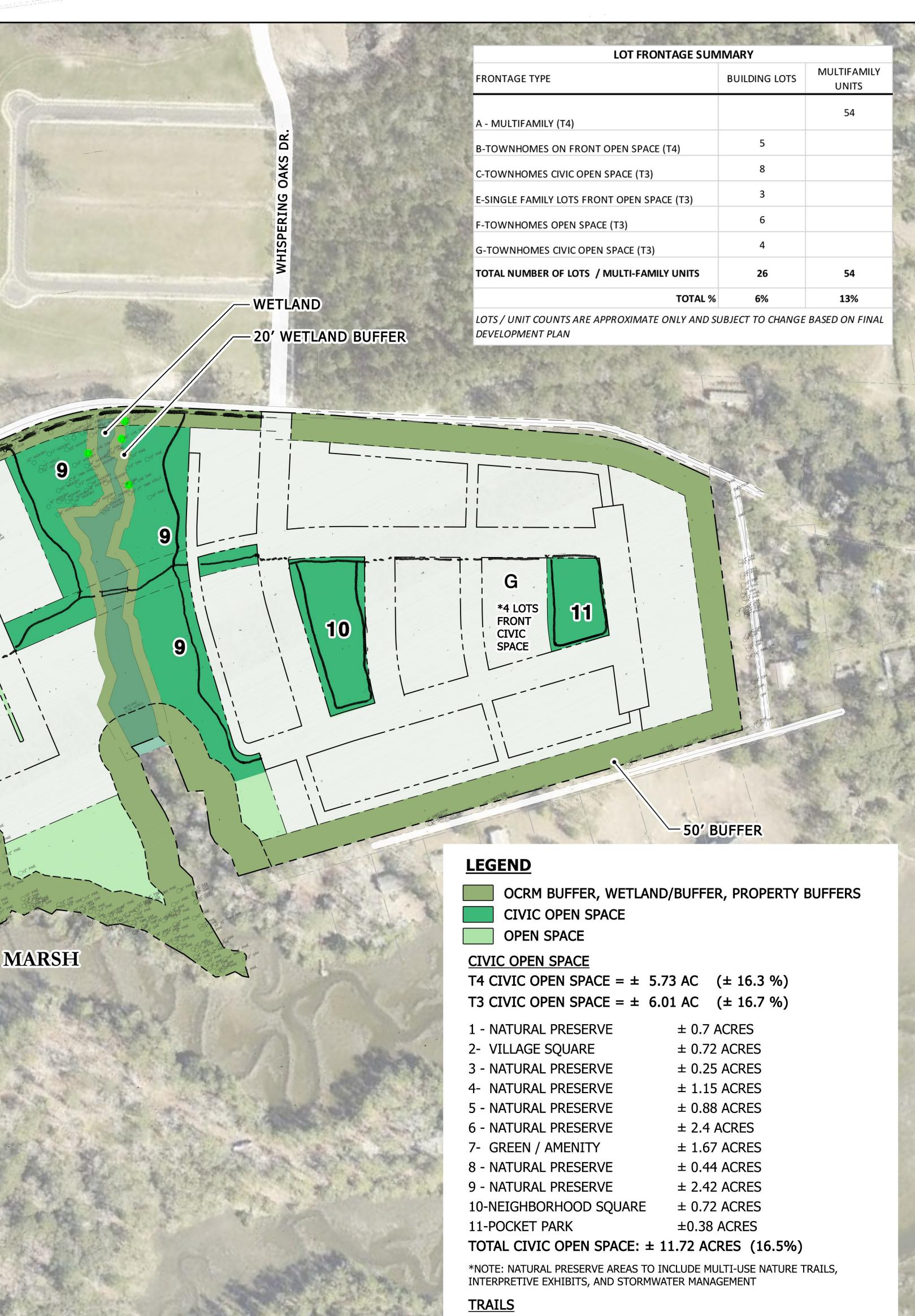
■ ■ ■ ■ HIGHWAY 170 MULTI-USE PATH (14' WIDE FUTURE BY BEAUFORT COUNTY - ASPHALT PAVING) - CHERRY POINT MULTI-USE PATH (8' WIDE-ASPHALT PAVING) - NEIGHBORHOOD NATURE TRAIL (5' WIDE - MINIMUM PERVIOUS SURFACE TO BE APPROVED AT TIME OF DEVELOPMENT PLAN SUBMITTAL)
