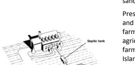
Diagram of a typical on-site sewage disposal system.
