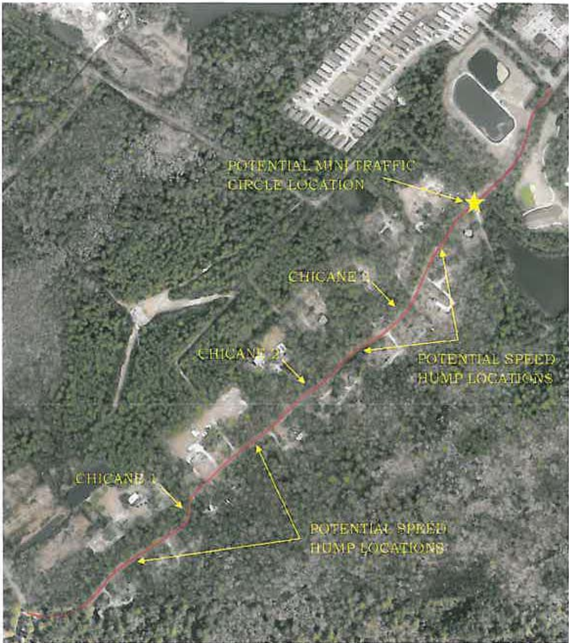
Figure 4.2 Potential Speed Hump and Mini Traffic Circle Location
