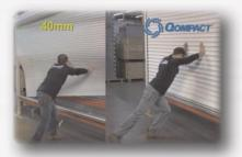
Qompact's end retention prohibits the curtain from being pushed out of the rails. Without end retention, the 40mm foamfilled curtain was easily compromised.
