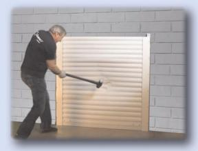
In impact testing, Qompact withstood 82 punches, 5 kicks, and 80 hits with a sledge hammer. The foam-filled shutter was destroyed in seconds.
