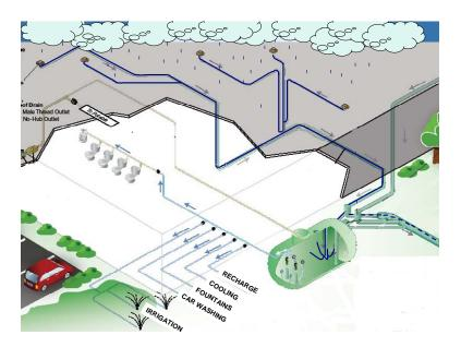
Figure 2b. Rainwater Harvesting System- Uses of Water Source: Rainfall Management Solutions – http://rainwatermanagement.com/
