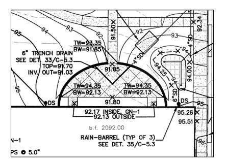
Figure 4. Details of stormwater management plan for Blacksburg Motor Company Building. *Source: Spectrum Design. "Blacksburg Motor Company Building Renovations C1.3."*
