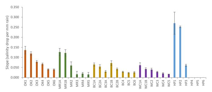
Figure 21. Slopes of equations for regressions of rain total (x) vs salinity drop (y). Huspah 4, 5, and 6 were not significant and are not shown (p > 0.2). All other regressions were significant except for May River 3 and 5 (p < 0.05).
