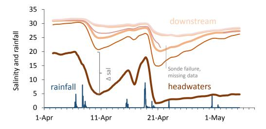
Figure 7. An example of filtered salinity data for all six Okatie River sites from two primary rain events in spring 2014. Darker colors represent more headwater sites, salinity response is dampened as the freshwater signal progresses downstream. An example of a salinity drop is brackted as  $\Delta$  sal for the first rain event.
