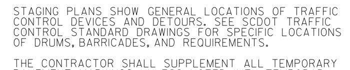
THE CONTRACTOR SHALL SUPPLEMENT ALL TEMPORARY PAVEMENT MARKINGS UNLESS NOTED WITH TEMPORARY RAISED PAVEMENT MARKERS THROUGHOUT THE PROJECT. PLACEMENT SHOULD BE AT THE DIRECTION OF THE ENGINEER.
